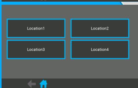
**Locations** – These are user calibrated measurements of parameters / surrogates that correlate to UV254 absorption. Such parameters as TOC, DOC, COD and BOD amongst others can be calibrated to UV254
