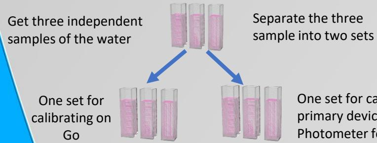
Perform the measurement of calibration parameter for example COD using the procedure from the manufacture of primary device.
